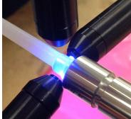
Image above is an example of catheter bonding using 3 poles.
